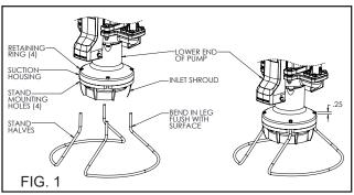
lower end. Push the stand legs into the pump lower end. Using a mallet, ensure that the stand legs bottom into the mounting holes. Repeat for the other stand half. Turn the pump upright on the installed stand.
