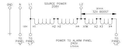
NOTE: PANEL "L1" IS THE ALARM CIRCUIT & PUMP RED WIRE PANEL "L2" IS THE PUMP CIRCUIT (THE BLACK WIRE) (REFER TO THE WIRING DECAL PROVIDED ON THE DOOR OF THE PANEL)
