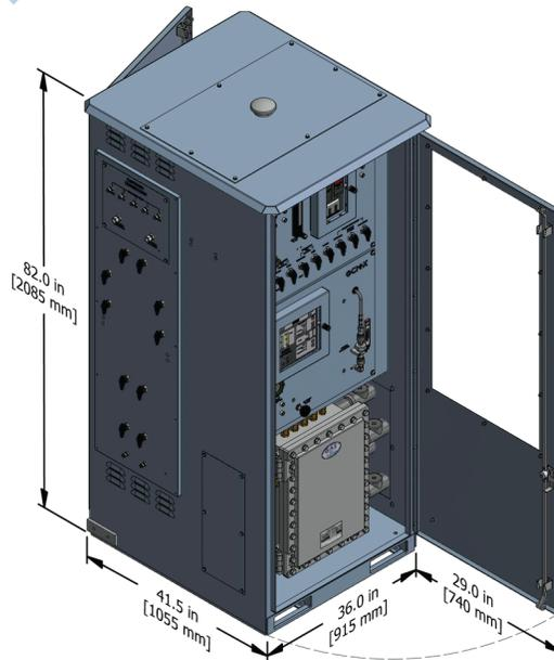
Door swing on NEMA enclosure is typical for both front and rear doors. Dimensions are for reference only and do not include recommended clearances. Contact E/One for detailed outline drawings.
