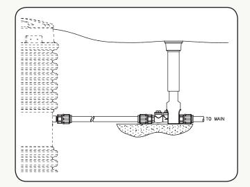
The UNI-LATERAL is a one-piece valve that can be installed between any grinder pump and the sewer main.
