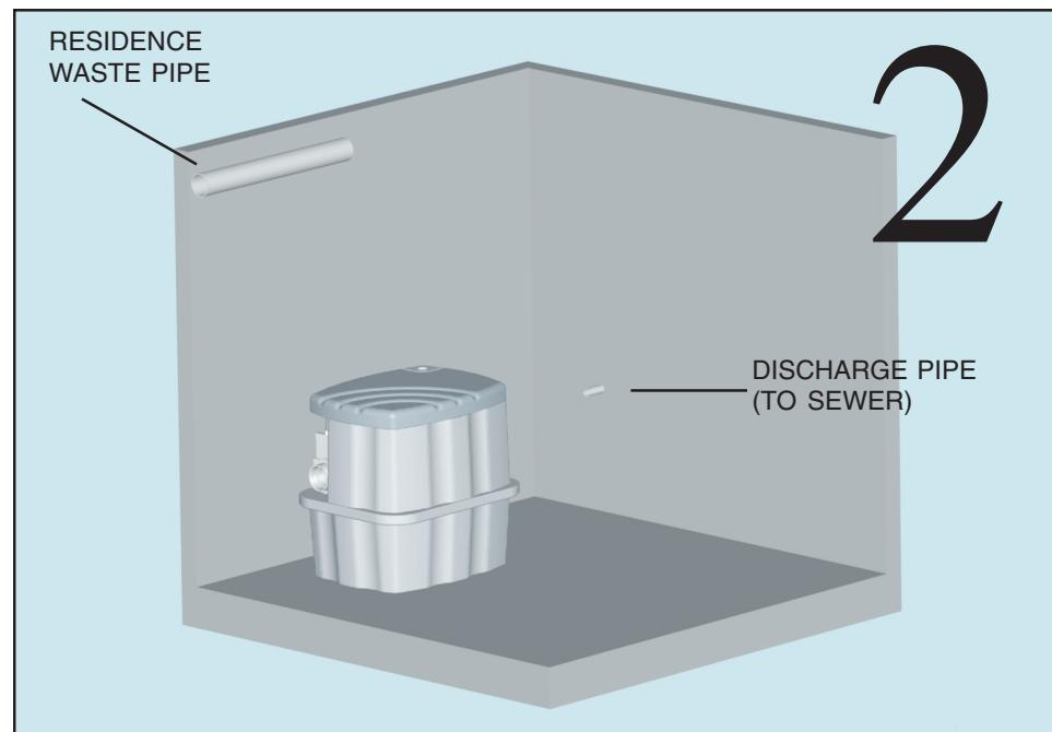
Place unit on basement floor, position based on the orientation of existing sewer/waste pipes. If the unit will be installed in an area where the alarm may not be seen or heard, the Remote Sentry Alarm Module should be installed.
