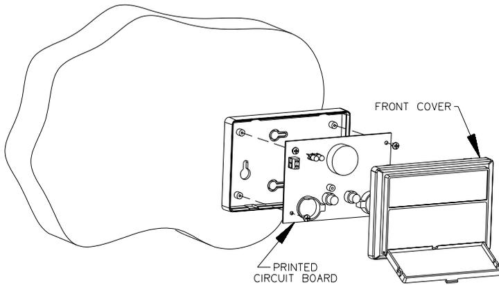
2. Disassemble the E/One Remote Sentry enclosure by snapping off the front cover. Remove the 4 screws securing the printed circuit board and remove circuit board.
