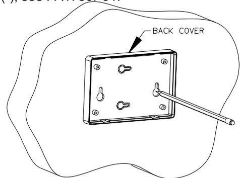
3. Mount the back cover to the wall. Run the cable through one of the holes in the cover. Do not connect the cable to the e|one Sentry yet.
