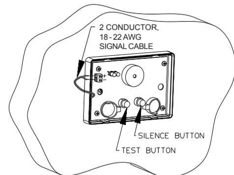
6. Press and hold the Test button. The E/One Remote Sentry Alarm LED will go on and the piezoelectric Buzzer will sound.
