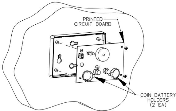
4. Remount the printed circuit board to the back cover.
